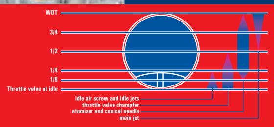
The above picture represents the choke and shows the influence of the different components as far as the throttle gas opening is concerned; it's just indicative and it's however a function of the combination of the different components and of the geometrical features of the conical needle.
