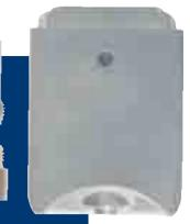
Another setting component is the **throttle valve**, which champfer influences more or less the idle and main circuit: higher is the component, more vacuum and flow speed will be reached with subsequent fuel increase on the intermediate and fast openings; therefore, by using throttle valves with a greater cut. we can get the contrary effect.
