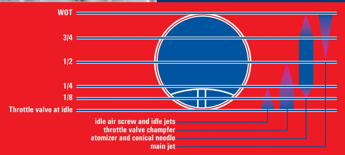
The above picture represents the choke and shows the influence of the different components as far as the throttle gas opening is concerned; it's just indicative and it's however a function of the combination of the different components and of the geometrical features of the conical needle.
