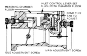
Be certain main diaphragm, gasket and cover casting are carefully fitted over the three small pins cast in rim at bottom of metering body; also the fuel pump gasket, diaphragm and fuel pump body, over similar pins at bottom rim of main diaphragm cover casting. Evenly tighten fuel pump body retaining screws to insure complete seal of casting separations at both diaphragms.
