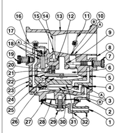
Note: On some models a one piece Idle Adjustment Screw (ref. 7) & Main Adjustment Screw (ref. 19) with rubberized "O" ring attached (not illustrated above) are used.
