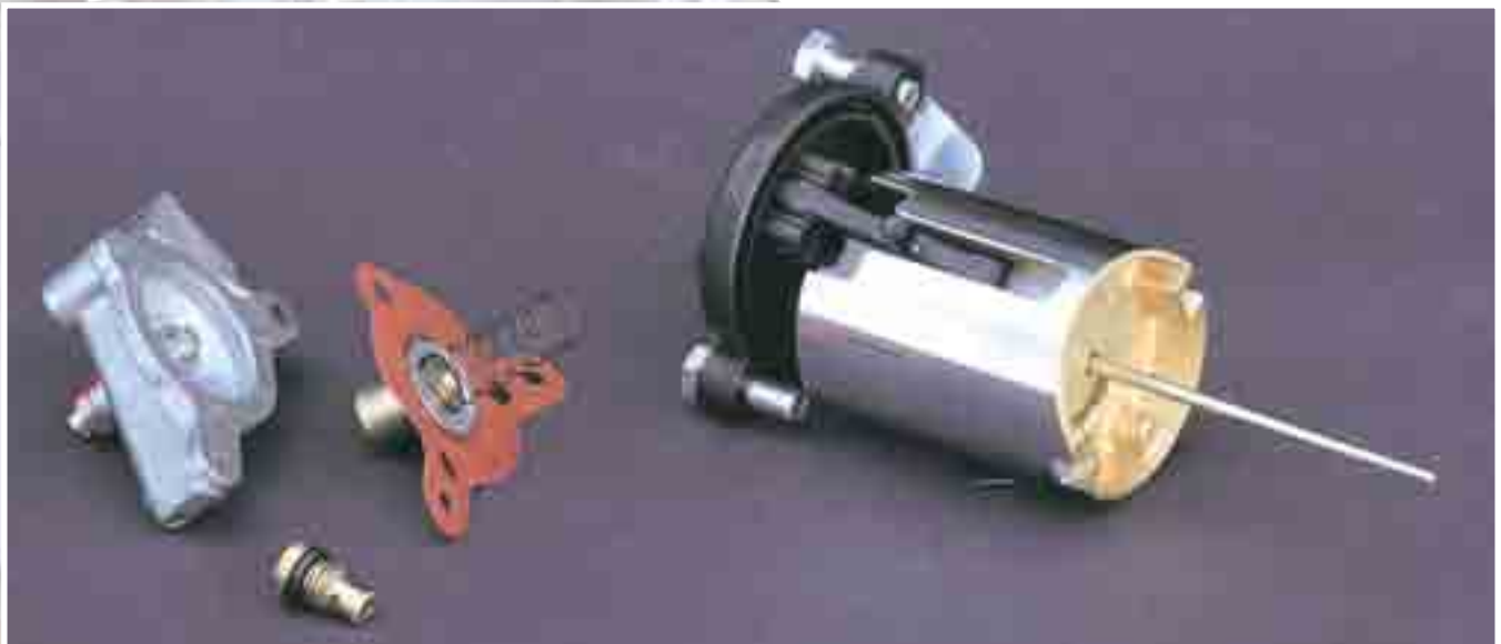
The acceleration pump fitted on a PHF carburetor and below, the same disassembled: we see the actual diaphragm pump and the lever system that is actuated by the inclined profile (cam) introduced in the Valve.
